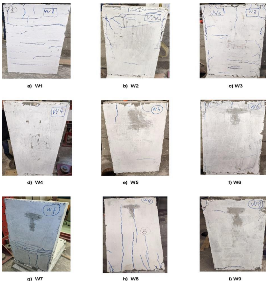
Figure 8: Tested Walls Crack Patterns.
