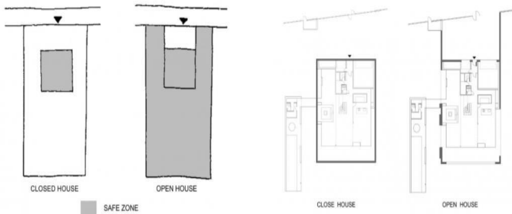
Figure 17: Conceptual and architecture plans showing the different between open and closed house in transformation of safe house.
