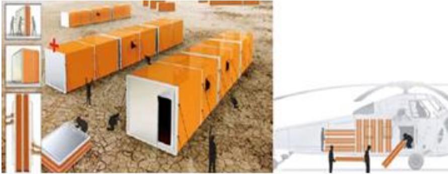
Fig. (12). Show the accordion tent shape and combined method when transporting
